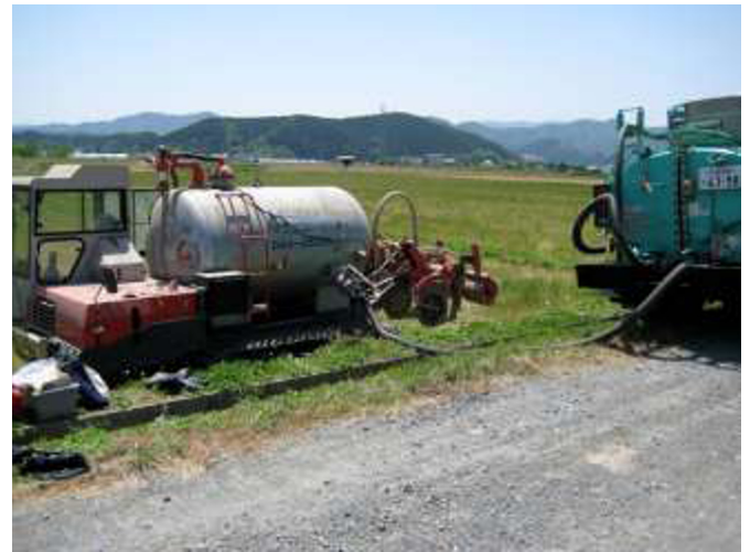
Fig. 3. Supplying liquid fertilizer from the vacuum truck to the slurry injector at the field in Nantan City.
