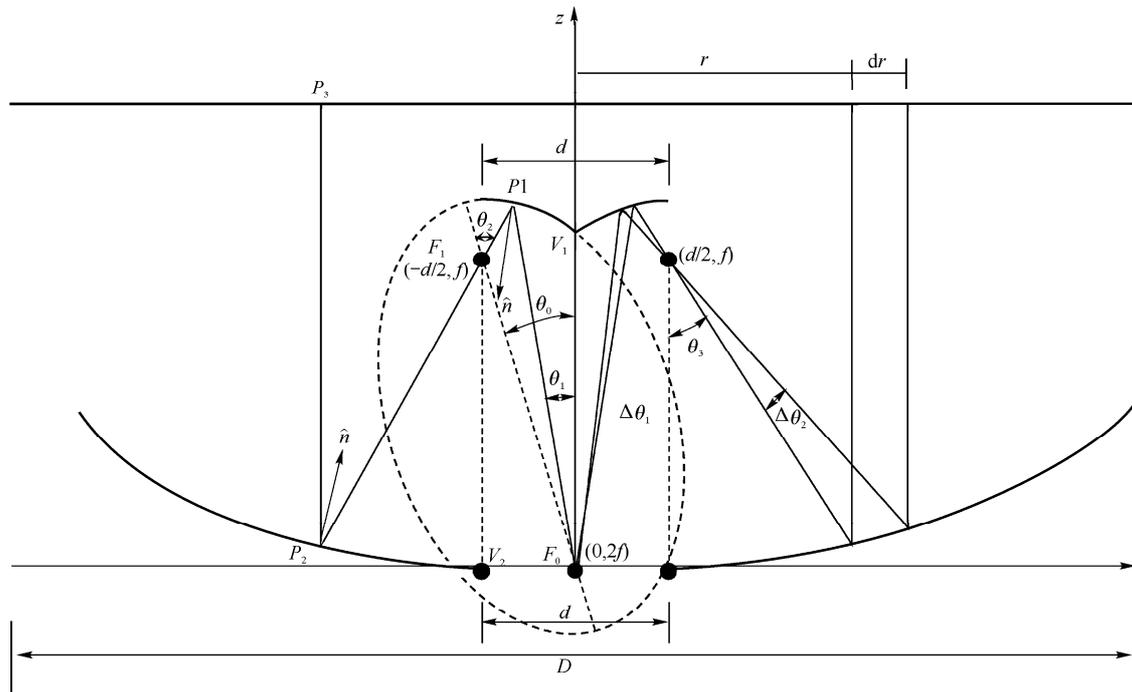
Fig. 1 The configuration of an ADE antenna and its parameters
