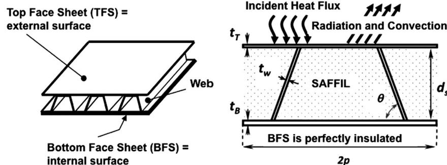
Fig. 1. Corrugated core sandwich panel ITPS concept.
