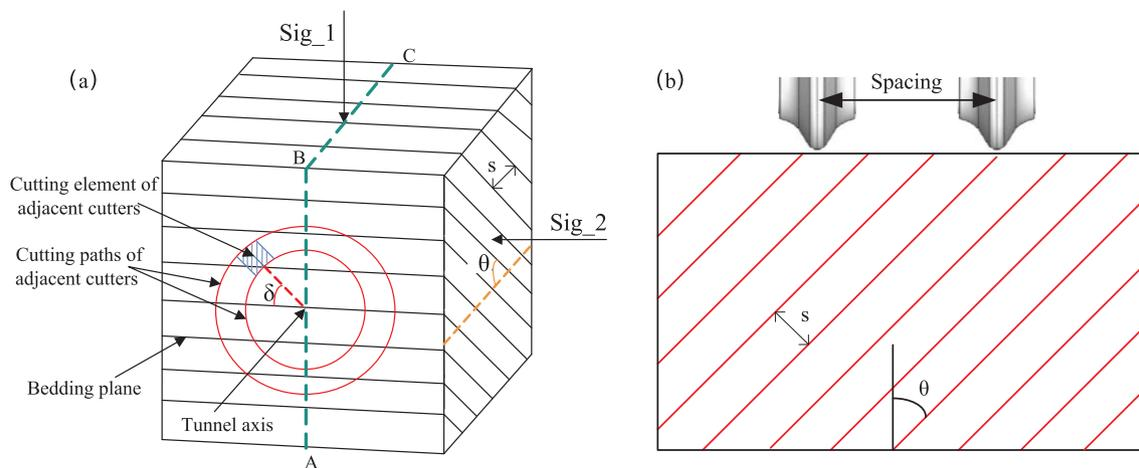
Fig. 1. Field and laboratory models: (a) a tunnel face in field; (b) previous studies of the chip formation in the ABC plane.
