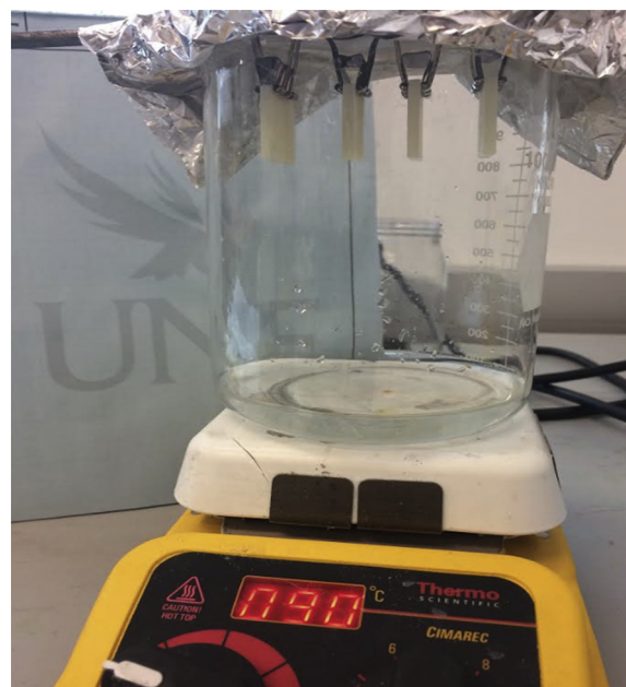
Fig. 2. Acetone Vapor Suspension. Acetone vapor surface treatment setup, showing the sample coupons suspended in a 1000 ml beaker with 100 ml of acetone at the base.
