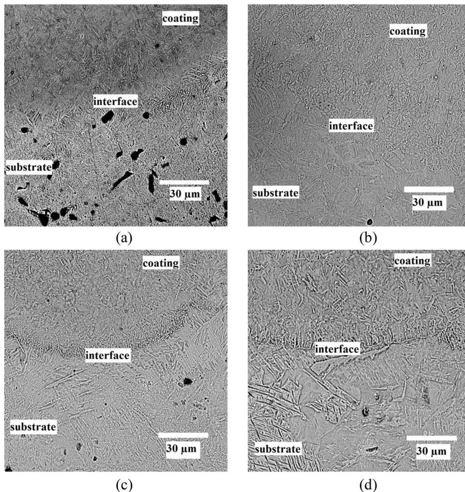
**Fig. 1.** Cross-sectional microstructures of composite coatings showing microstructural features and diffuse interface (a) BG200, (b) BG300, (c) HA200, (d) HA300.
