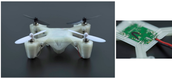
Fig. 1. FDM printed functional quadcopter. Printed via Voxel8 with embedded electronics and endures structural loading [4].
