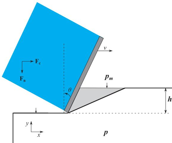
Fig. 1. Geometric model of the rock cutting process.
