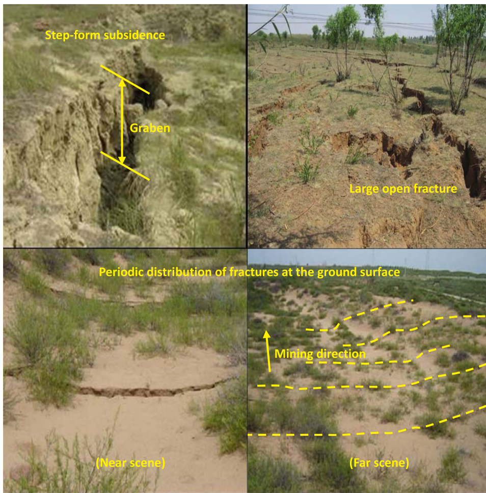
Fig. 1. Surface fracture distribution after longwall mining.
