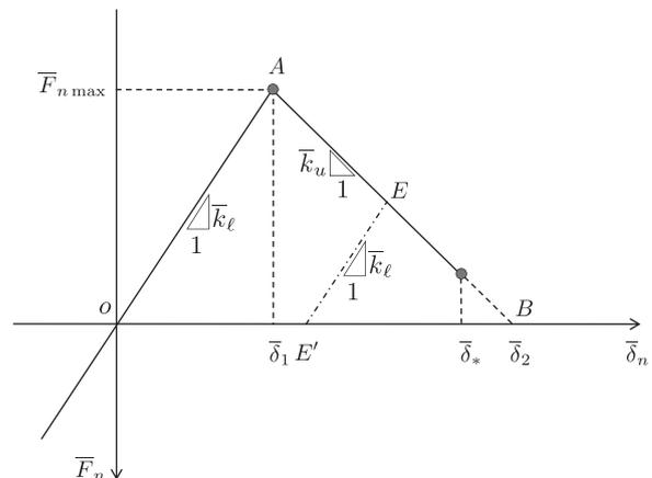
Fig. 1. Normal force-displacement contact law for the parallel bond.
