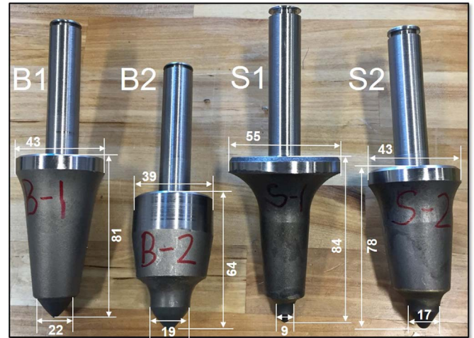
Fig. 3. Engineered conical cutting bits within ± 2 g of deviation. B1: BETEK coal cutting bit; B2: BETEK rock cutting bit; S1: Sandvik coal cutting bit; and S2: Sandvik rock cutting bit. Unit is millimeter (mm).
