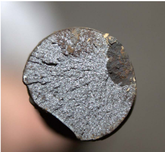
Fig. 1. Photograph of an SCC failure surface on a rockbolt recovered from an underground coal mine in NSW, Australia.
