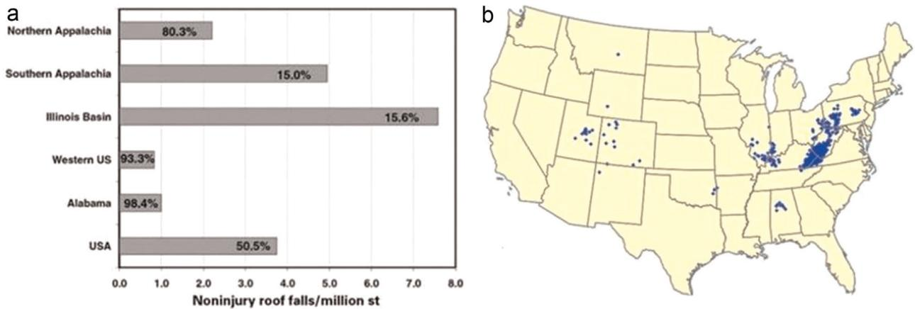
Fig. 1. (a) Roof fall rate in U.S. coalfields from 2005–2006.<sup>11</sup>Note: Percentage in bars indicate the percent of production due to longwall mining method, and (b) location of active underground coal mining operations, 2012.<sup>10</sup>
