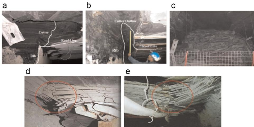
Fig. 2. Stages of “cutter-roof” failure development (a) initial stage of a cutter, (b) small cutter type roof fall at a corner, and (c) roof profile after a massive fall initiated by cutters. Photo credits: Murali Gadde and SS Peng.<sup>6</sup>
