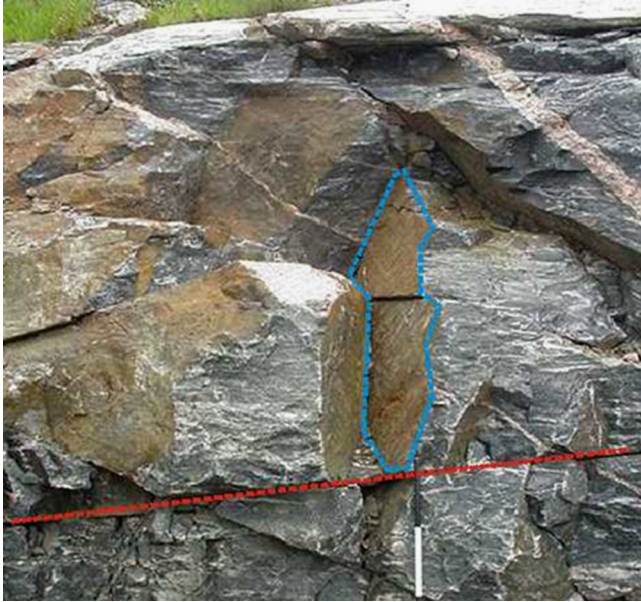
Fig. 1. Rock cut showing both fracture trace (red line) and facet (cyan polygon) [7].
