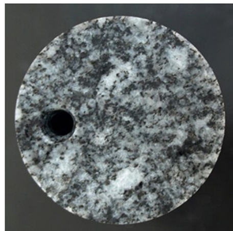
Fig. 1. Rock sample preparation (mm) for permeability test.
