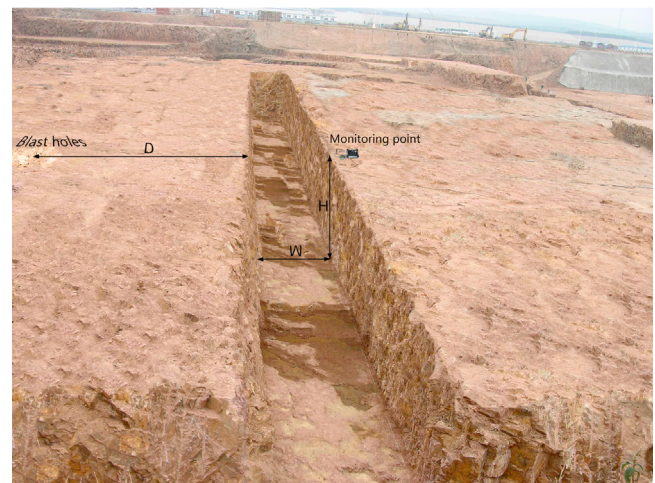
Fig. 2. Blast vibration measurements in sites with different topographic features. (a) Upward slope site. (b) Damping ditch site.
