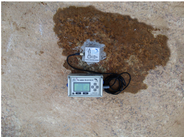
Fig. 1. Vibration sensor and data logging instrument of the vibration monitoring system.
