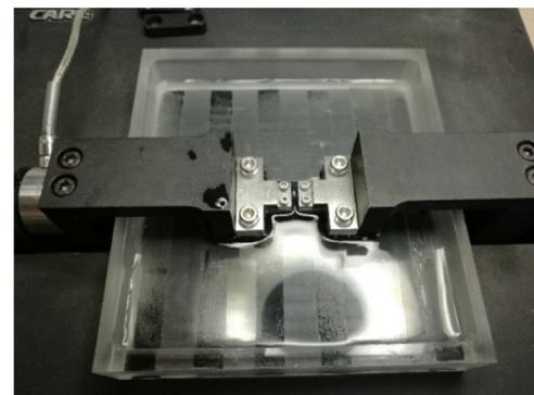
Fig. 3. Photograph of in-situ micro tension cyclic testing system.
