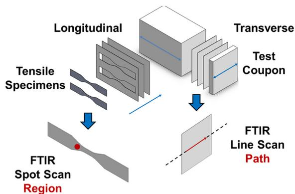
Fig. 1. Sectioned 5 × 5 × 8 cm rectangular prism sample. Tensile specimens stamped from microtomed thin sections (longitudinal side) along with FTIR spot scan region; FTIR line scan path on thin section from test coupon (transverse side).
