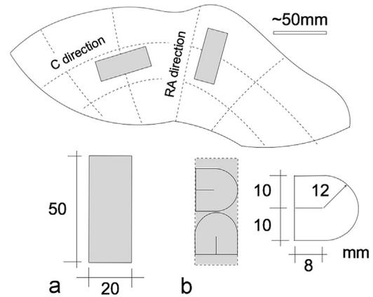
**Fig. 1 – a) Rectangular samples. b) Tear geometry. Cut length: 8mm. Radius: 12 mm. RA (root-to-apex), C (circumferential).**
