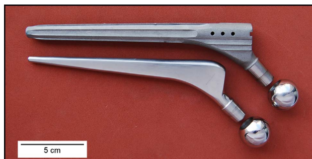
Fig. 1 – Modular hip prostheses: Model SS/Ti Cemented (top) – head made of ASTM F138 stainless steel and stem made of ASTM F136 Ti-6Al-4V alloy; Model SS/SS Cementless (bottom) – head and stem made of ASTM F138 stainless steel.
