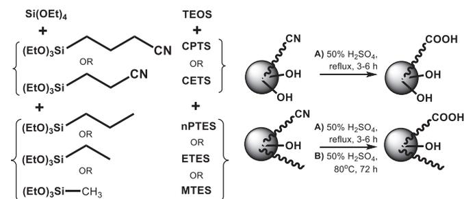
**Fig. 3.** Co-condensation of TEOS, cyanosilanes, and various alkyl silanes to yield solid particles. Nitriles are converted to carboxylates by route A), reflux in  $\text{H}_2\text{SO}_4$  for 3–6 h, or, route B), heating in  $\text{H}_2\text{SO}_4$  for 72 h at 80 °C. Total organic surface densities range from 1 to 5  $\text{nm}^{-2}$ , with up to 77% conversions to peracid.
