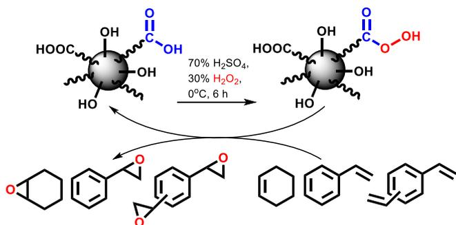
**Fig. 1.** Generalized synthesis of peracids from the corresponding grafted carboxylate in  $\text{H}_2\text{O}_2/\text{H}_2\text{SO}_4$  and their use, in a second step, as epoxidation agents for cyclohexene, styrene, or divinylbenzene.
