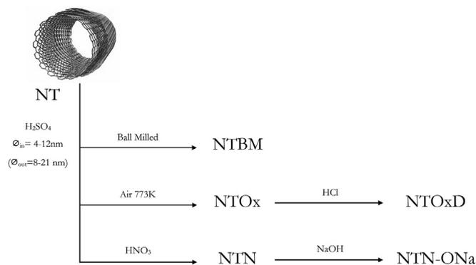
Fig. 1. Preparation of supports.
