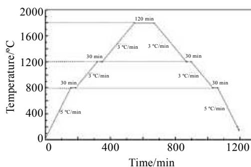
Fig.2 Sintering temperature and holding time of liquid phase sintering (LPS)
