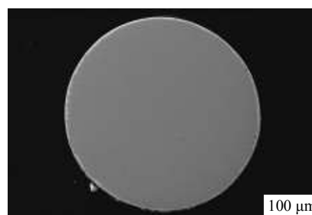
Fig.1 Cross-section photograph of Zr_{41.2}Ti_{13.8}Cu_{12.5}Ni_{10}Be_{22.5} BMG-coated Q195 steel wire
