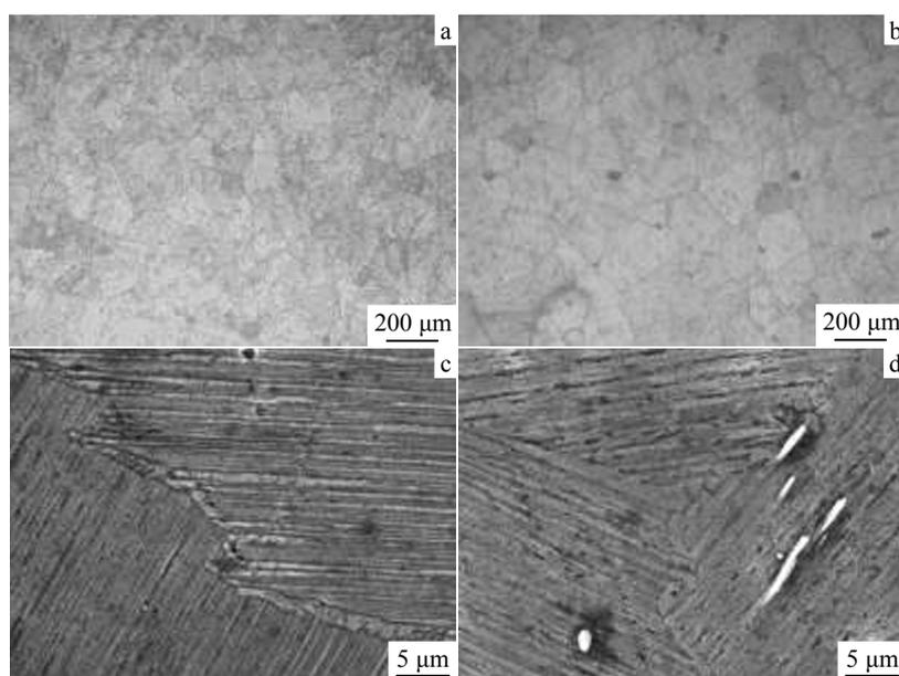
Fig.1 OM (a, b) and SEM (c, d) of microstructures of TiAl alloys: (a, c) small lamellar colony and (b, d) large lamellar colony
