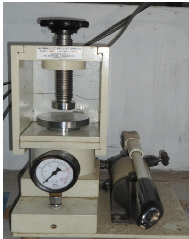
Figure 1 Photographic view of manually operated hydraulic pelletizer.
