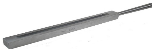
Fig. 1. Metallic strip ingot mould used.
