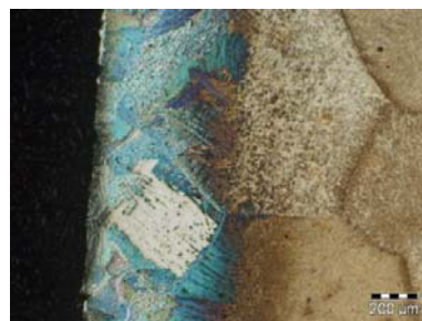
Fig. 1. Ti10V2Fe3Al alloy microstructure, alpha case on sample's surface (left layer), etched with Kroll's reagent [5].
