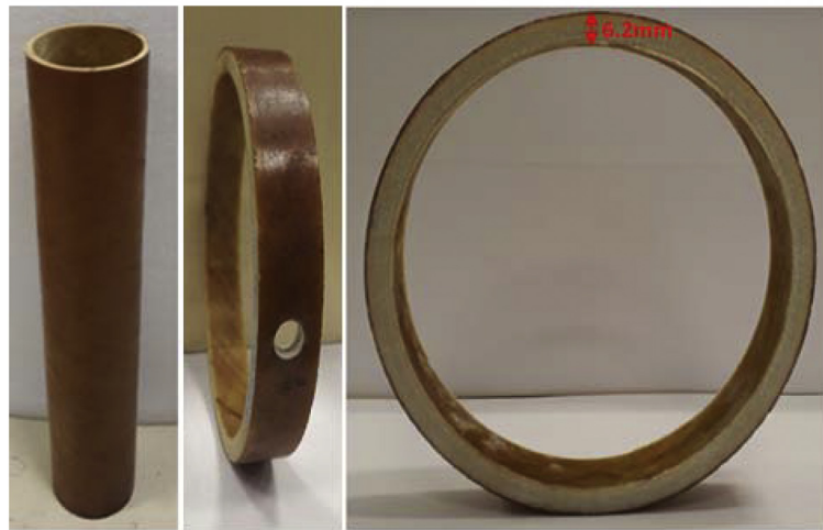
(b) Tested polymer pipe specimens
