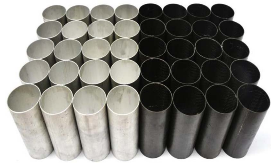
Fig. 1. Specimens before quasi-static axial and oblique compression test.
