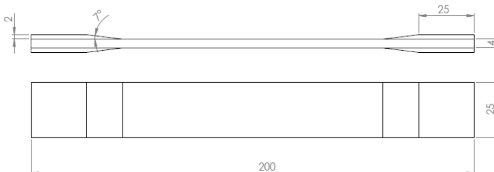
Fig. 3. Tensile test specimen according to ASTM D3039.
