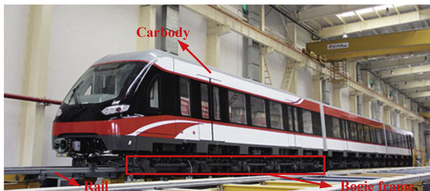
Fig. 1. Medium-low maglev train produced by CRRC Zhuzhou Electric Locomotive Co., Ltd.
