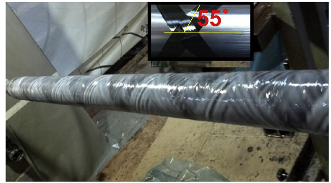
Fig. 1. Filament winding process of carbon fiber/epoxy composite pipes. The inset represents winding angle as \pm 55^\circ .
