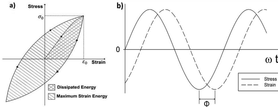
Fig. 1. a) Hysteresis curve for a non-linear material [8] and b) cyclic stress and strain [9].
