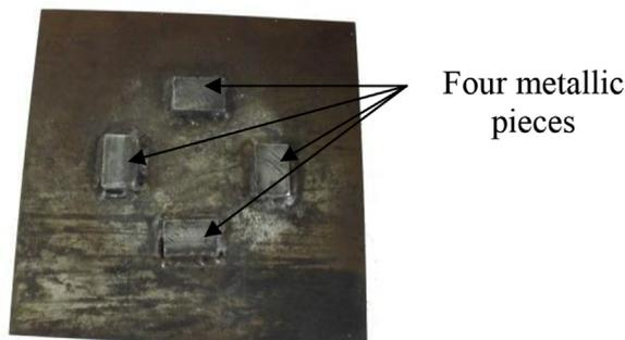
Fig. 1. Four-piece metallic trigger located on a flat plate.
