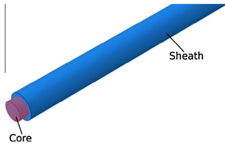
Fig. 1. Structure of core/sheath type bi-component fibre.
