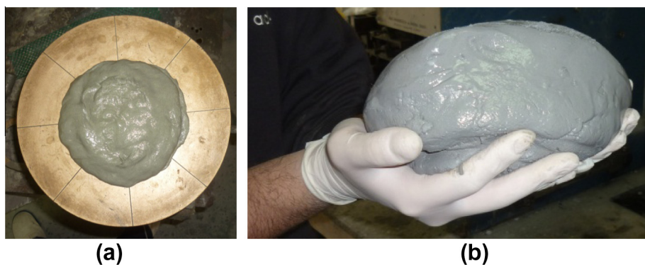
Fig. 1. The spread diameter of PP fiber reinforced MI matrix (a) and deformability of PP fiber reinforced MIII matrix incorporating SBR latex emulsion (b).
