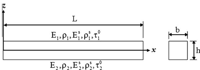
Fig. 1. Geometry of a FG nanobeam.
