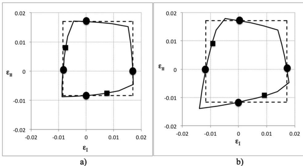
Fig. 2. Omni strain LPF envelopes for two CFRPs based on Tsai-Wu (solid line) and maximum strain (dashed line). a) IM7/977-3; b) T700/2510.
