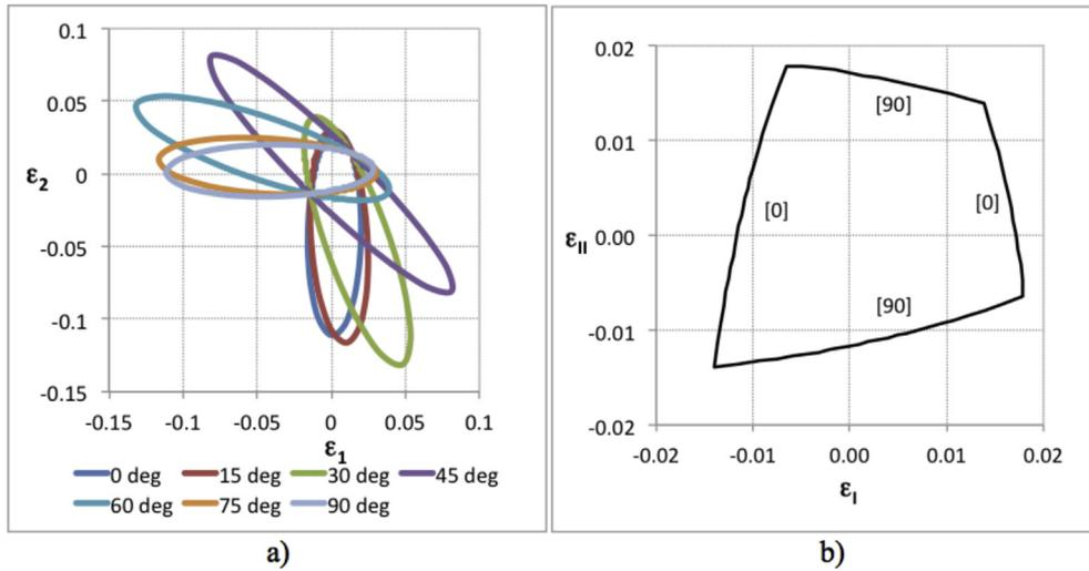
Fig. 1. a) Superposition of LPF envelopes for T700/2510 using Tsai-Wu with  $F_{xy}^* = -1/2$  and  $E_m^* = 0.15$ . b) Omni strain LPF envelope for T700/2510.
