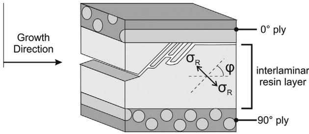
**Fig. 1.** Delamination growth in mixed-mode delamination starting at the interlaminar resin layer in a 0°/90° ply interface [5]. The angle  $\phi$  at which the microcracks develop is dictated by the resolved stress ( $\sigma_R$ ) in the interlaminar resin layer near the crack tip.
