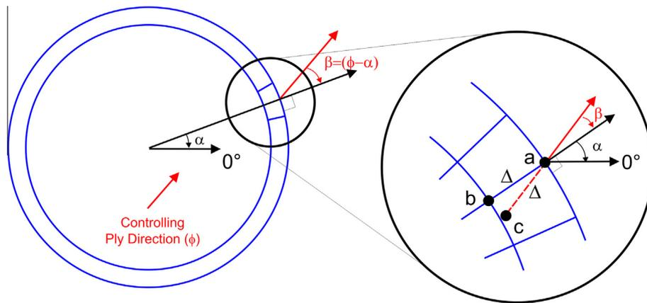
**Fig. 2.** Redefined nodal position for determining  $G_{II}$  and  $G_{III}$  [7]. While  $\alpha$  defines the orientation of the crack front, crack growth depends on the orientation of the directing ply, defined by  $\phi$ , and their mismatch  $\beta$ . The points  $a$  and  $b$  are nodes in the FE mesh, point  $c$  is a point defined in this figure, all used for VCCT calculations.
