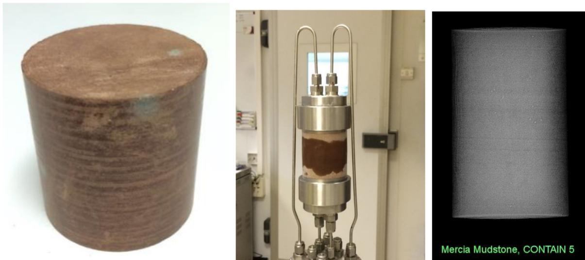
**Fig. 1.** A sample of Mercia Mudstone after preparation (left), arranged within the isotropic test assembly (centre) and as a 2D x-ray image (right).
