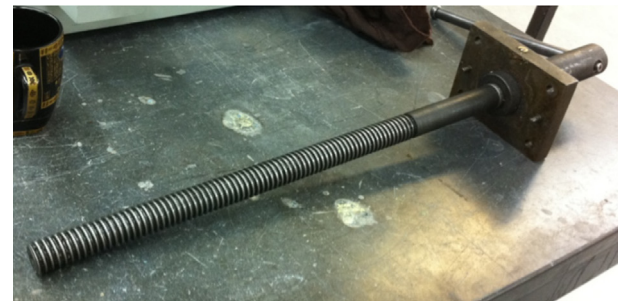
(b) Deformed power screw
