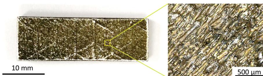
**Fig. 1.** As-printed CoCrFeMnNi HEA sample.
