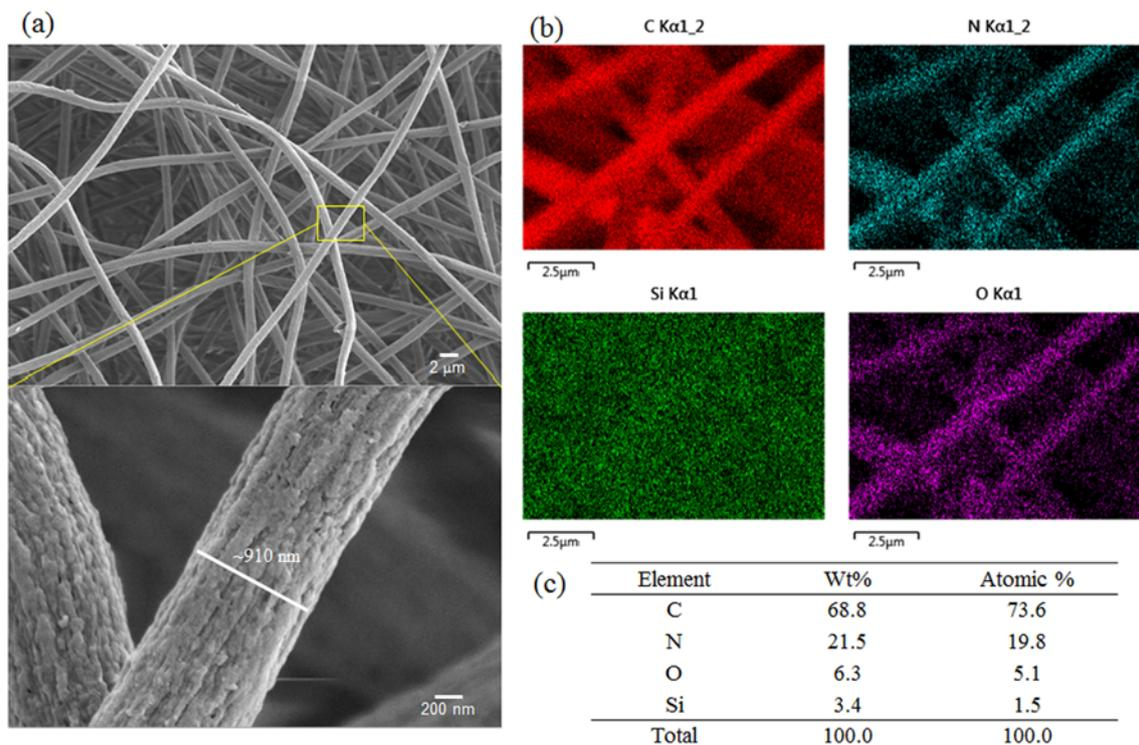
Fig. 1. (a) SEM images, (b) elemental mapping images, and (c) relative elemental composition of as-electrospun precursor nanofibers with 40 wt% POSS.
