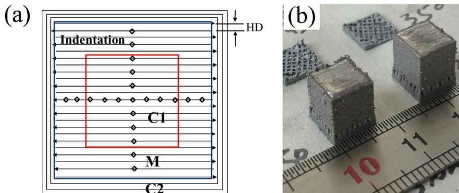
Fig. 2. the schematic illustration of (a) laser trace mode with indenter (C1 = Center, M = Middle, C2 = contour) and (b) the SLM-processed samples.
