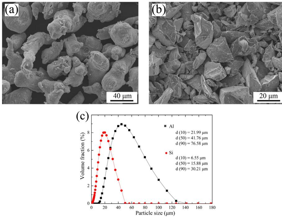
Fig. 1. SEM images of the morphology of powders (a) aluminum, (b) silicon and (c) their size distributions.
