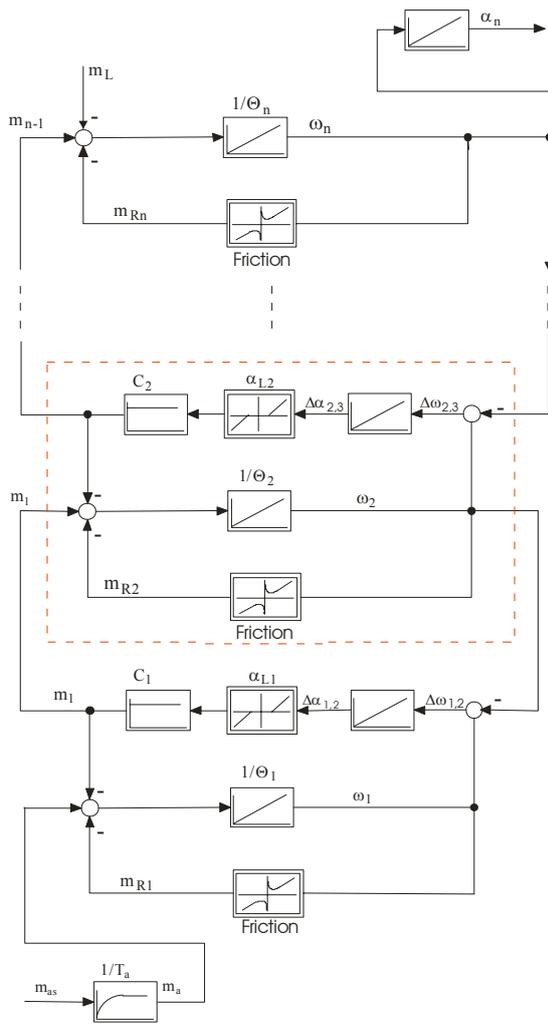
Fig 2: Block diagram of a multi mass system
