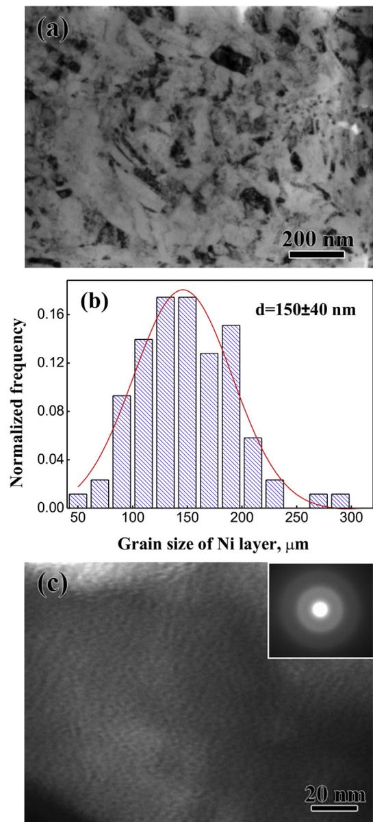
**Fig. 1.** Microstructure characterization of sandwich-structured UFG-Ni/Fe<sub>78</sub>B<sub>13</sub>Si<sub>9</sub> amorphous alloy/UFG-Ni composite, (a) TEM cross-sectional image of UFG-Ni layer; (b) distribution of grain size of UFG-Ni layer, (c) TEM image of Fe-based amorphous ribbon.
