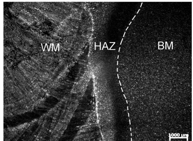
**Fig. 2.** Partial outline of welded joint with heat input of 1.43 kJ/mm.
