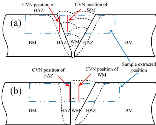
**Fig. 1.** Schematic diagram showing double (a) and single (b) bevel V-type groove preparation. The extracted position of cross weld samples and CVN position are signified with arrows.
