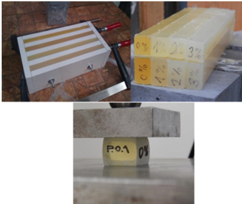
Fig. 1. Compression test sample preparation and testing process.
