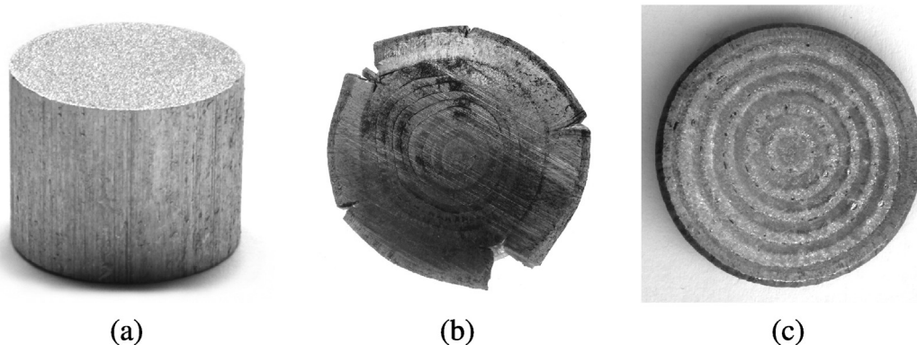
Fig. 2. Compression test specimens; (a) before testing (outside diameter = 12.7 mm), (b) after testing on an ambient extruded sample, and (c) after testing on an evacuated extruded sample.
